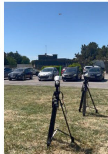
Dual axis motorized antenna with tracking capabilities
