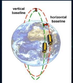
Definition: A 3D satellite formation that combines out-of-plane (horizontal) orbital displacements (by relative inclination vector) with in-plane (vertical) orbital displacements (by relative eccentricity vector).
