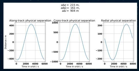
• Selecting ∂≠90° introduces a difference in the orbital inclination between the two Harmony satellites.
