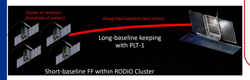
Vertical and cross-track separations together with significant along-track drift wrt PLT-1 allowed and managed within DSAR image generation
