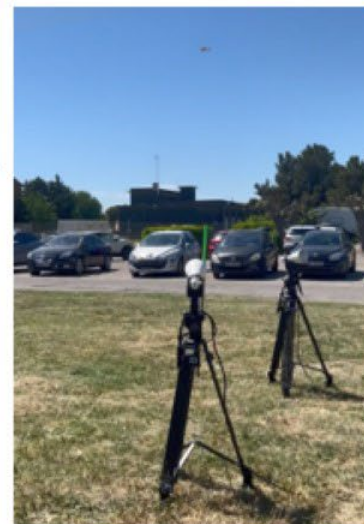
Dual axis motorized antenna with tracking capabilities
